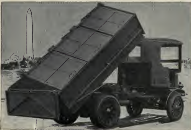
GARBAGE COLLECTION TRUCK IN DUMPING POSITION
